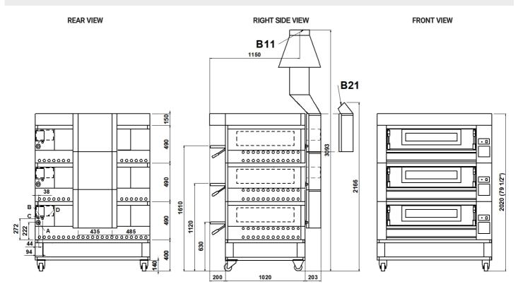
NOTE: The dimensions indicated in the views are in millimeters. B11 DIRECT VENTILATION (ø int 254mm). B21 UNDER VENTILATION HOOD
